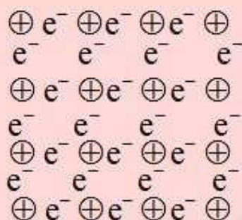
Fig. 2.1. Electron sea model of metal.
