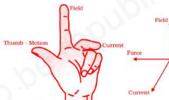
Figure 9.16 Fleming's Left-Hand rule
