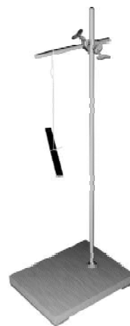
Fig. 13.9 A freely suspended bar magnet always comes to rest in the same direction
