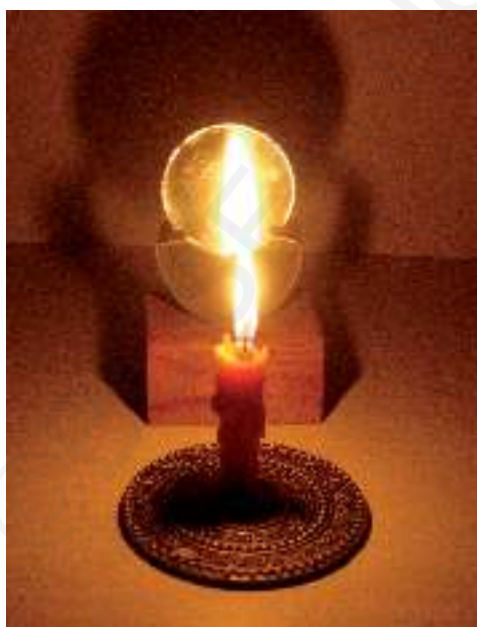
Fig. 15.16 Virtual image formed by a concave mirror
