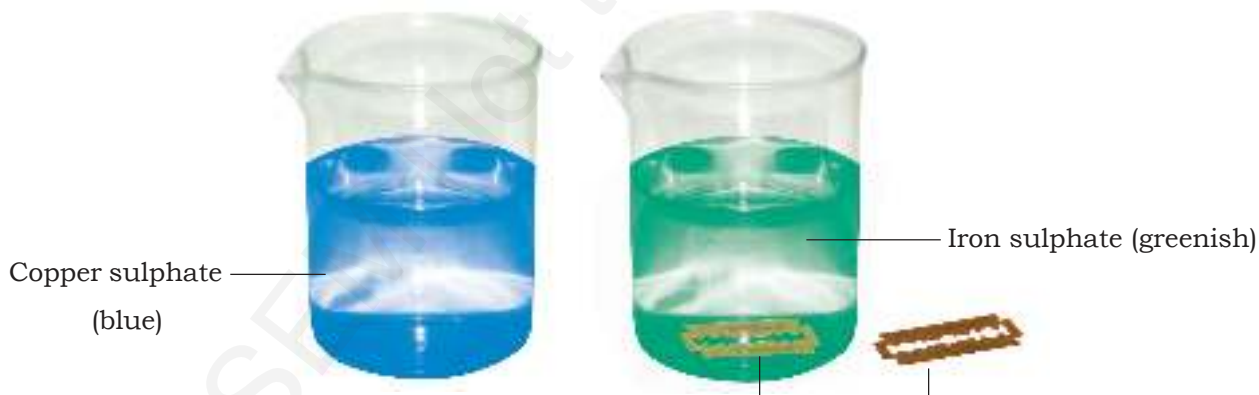
Fig. 6.4 Change in colour of the copper sulphate solution due to reaction with iron
