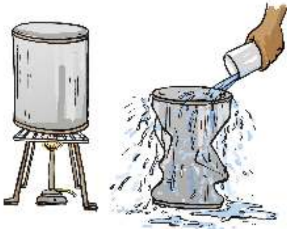
Fig. 8.2 Can with hot water being cooled
