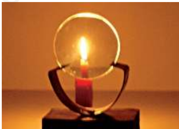
Fig. 15.27 Image formed by a concave lens
