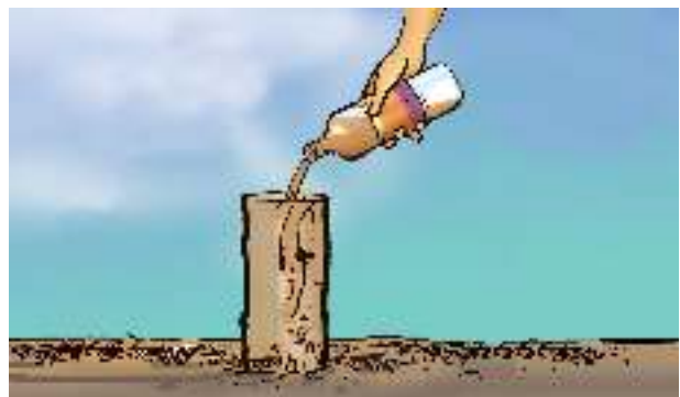
Fig. 9.5 Measuring rate of percolation
