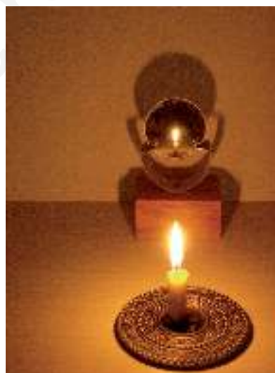
Fig. 15.19 Image formed by a convex mirror
