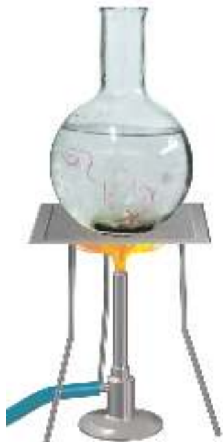
Fig. 4.9 Convection of heat in water
