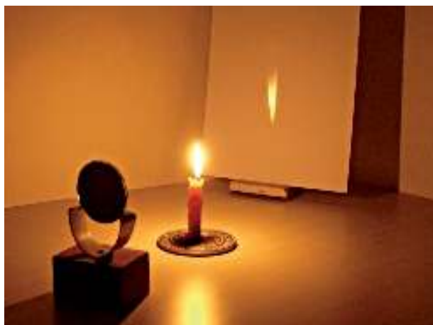
Fig. 15.15 Real images formed by a concave mirror
