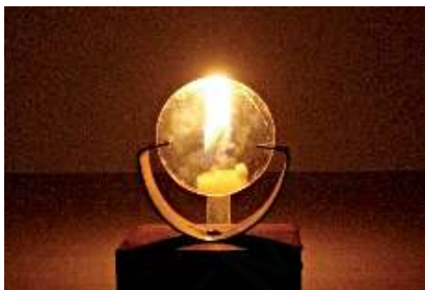
Fig. 15.26 Virtual image formed by the convex lens
