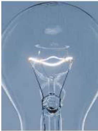
Fig. 14.12 Glowing filament of an electric bulb (incandescent)
