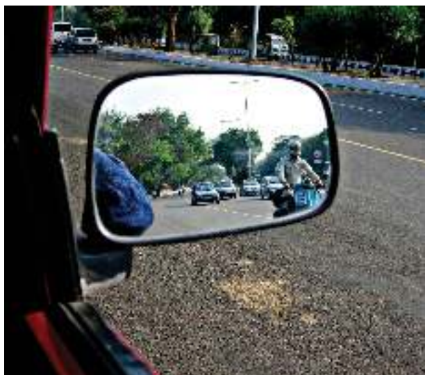
Fig. 15.20 Convex mirror as side view mirror
