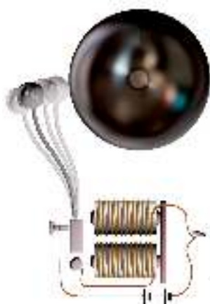
Fig. 14. 20 Circuit of an electric bell
