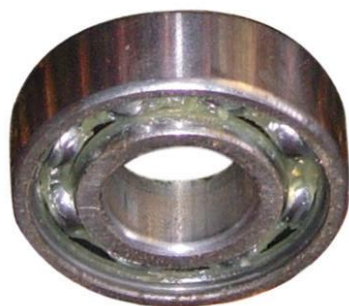
Fig. 12.16 : Ball bearings reduce friction
